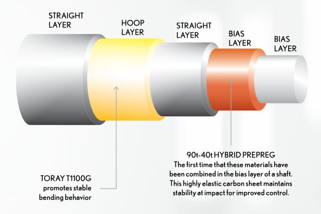
Miyazaki test data shows that the new shaft construction has 6 percent lower face angle dispersion at impact and 12 percent lower dispersion of loft angle at impact.
